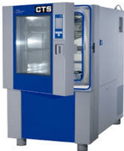
Figure 3: Fondazione OMD Climatic chamber (left), and WXT520 Calibration using three PT100 as transfer standards (right).
