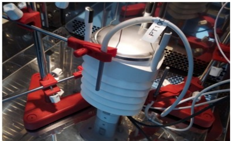
Figure 3: Fondazione OMD Climatic chamber (left), and WXT520 Calibration using three PT100 as transfer standards (right).
