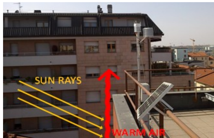
Figure 6: Upward flow of warm air from underlying wall in MI Bovisa station
