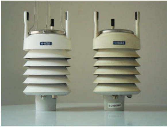
Figure 1. Photograph of two of the AWSs used in the field trial. Left: 1 years old AWS (AWS1), in the right: 3-year-old device (AWS3). It is evident the colour variation of screen coating due to the ageing.
